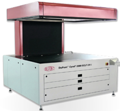
Figure 2: Exposure unit with dimmable lamps
